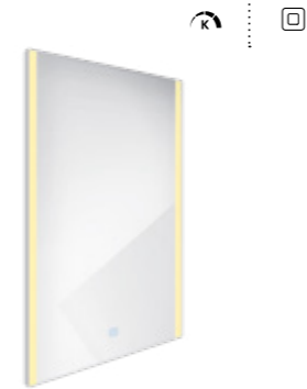
LED mirror 500 x 700 With touch sensor. Possibility of setting the color temperature 2700K - 6000K. Output 21W. Aluminium frame.
