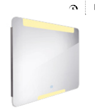
LED mirror 800 x 700 With touch sensor. Output 16,5W. Possibility of setting the color temperature 2700K - 6000K. Aluminium frame.
